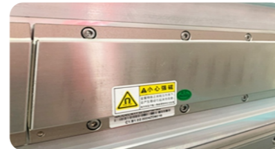
Linear motor for more accurate and stable moving on X axis (Optional)
